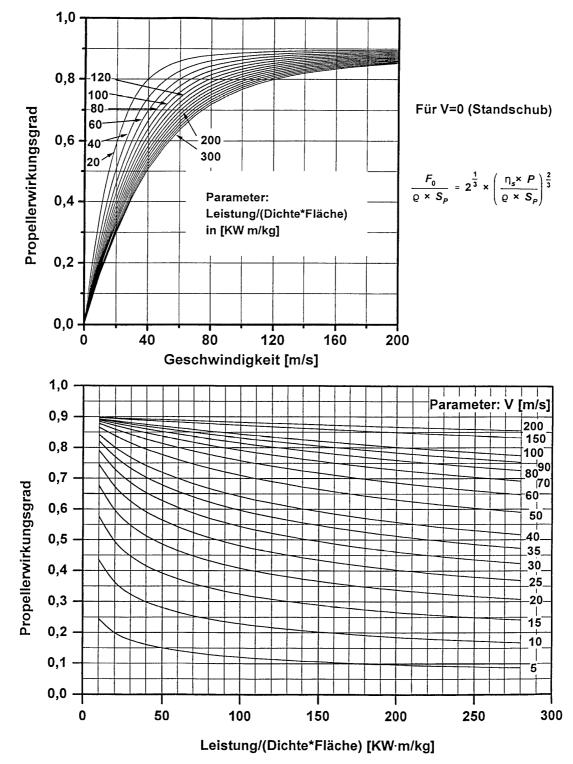
**Figure 5** Propeller efficiency (Propellerwirkungsgrad) as function of aircraft speed (Geschwindigkeit). Parameter used is shaft power (Leistung) devided by air density (Dichte) times propeller area (Fläche). For the aircraft with V=0 a separate equation is provided to calculate the thrust at rest
