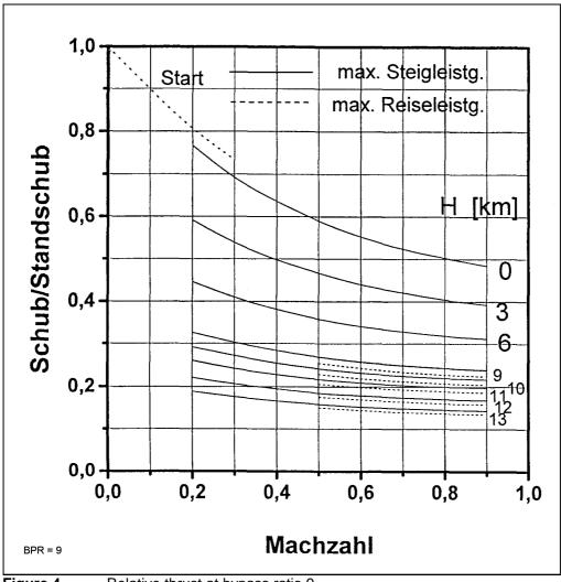
Figure 4 Relative thrust at bypass ratio 9
