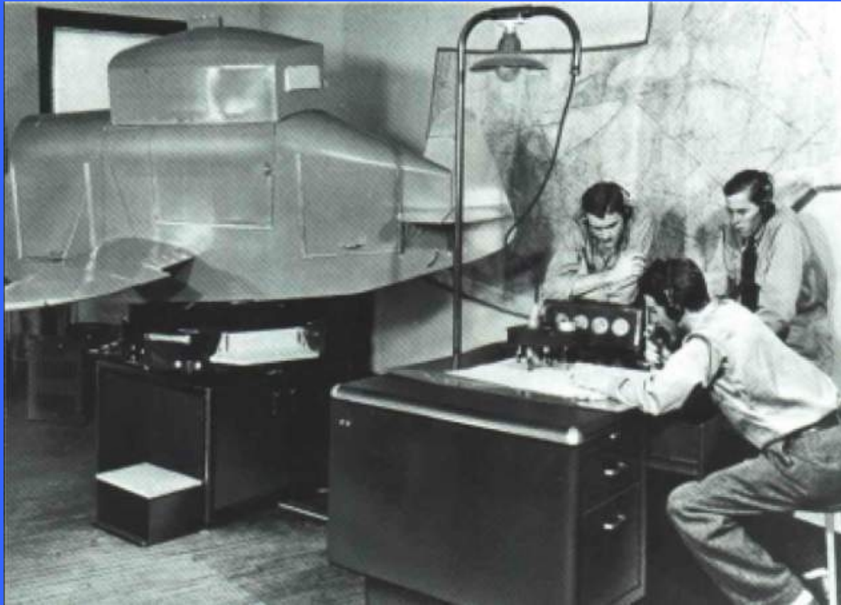
1940 Link Trainer Instructor Operating Station Run by the instructor outside the cockpit No View of Pilot's Operation – not suitable for assessing multi crew operation
