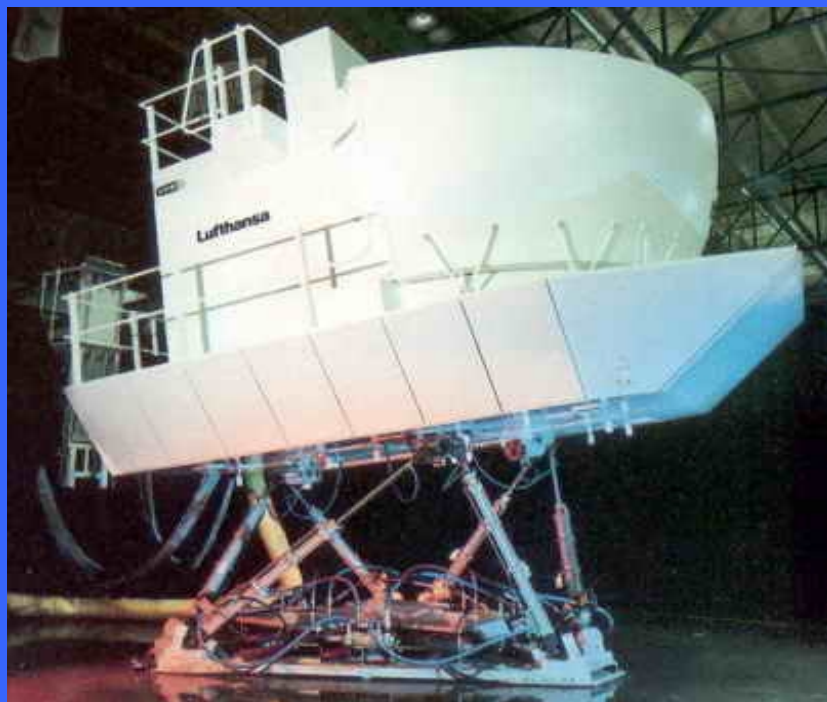
Current Simulators also have Motion and Visual Systems 1998 CAE A340 at Lufthansa Flight Training
