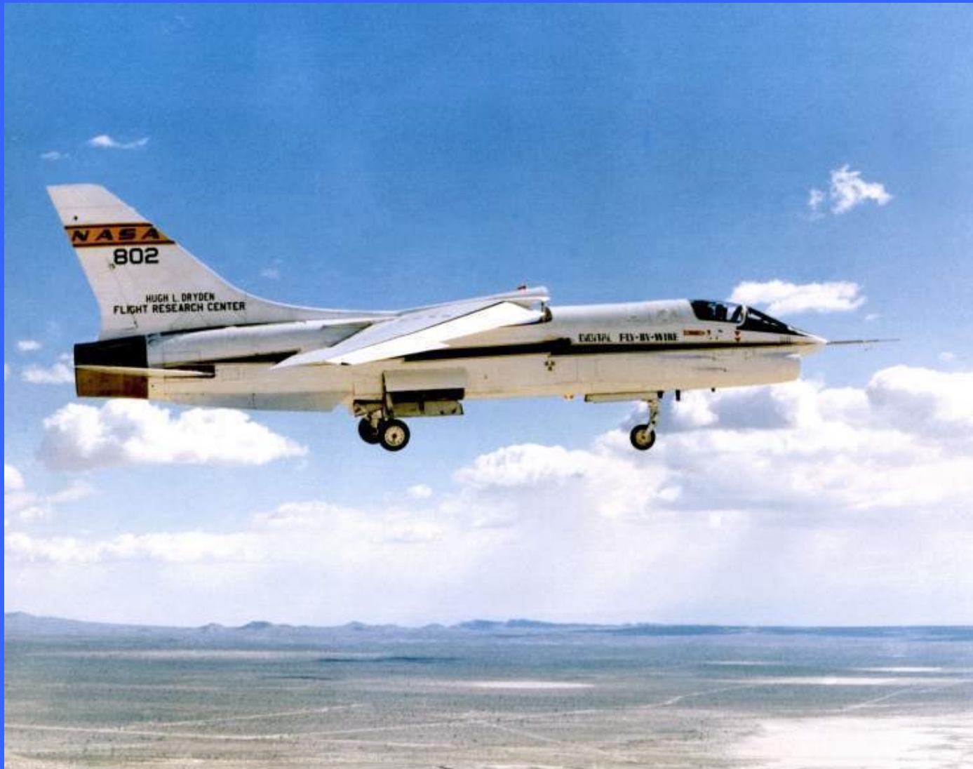
Dryden Flight Research Center EC77-6988 Photographed 1977 F-8 DFBW (Digital Fly-by-Wire) contributed vastly to systems aboard the Space Shuttle. NASA Photo
