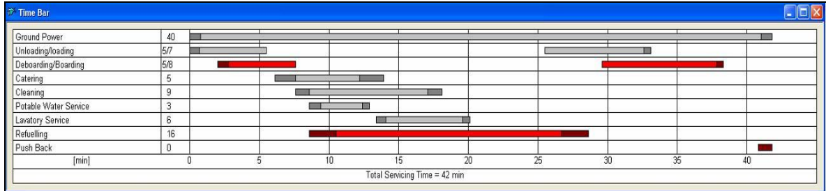
Figure 12.2 SIMBA time bar chart of the reference aircraft simulation
