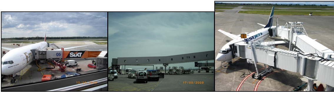
Figure 2.2 Passenger boarding bridges (left and centre) and bridge OTW (right) ( Dewbridge 2009 )
