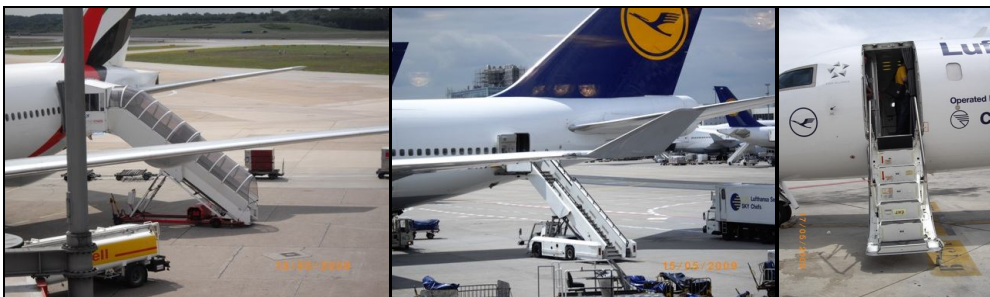
Figure 2.3 Manually stair (left), stair truck (centre) and integrated stair (right)
