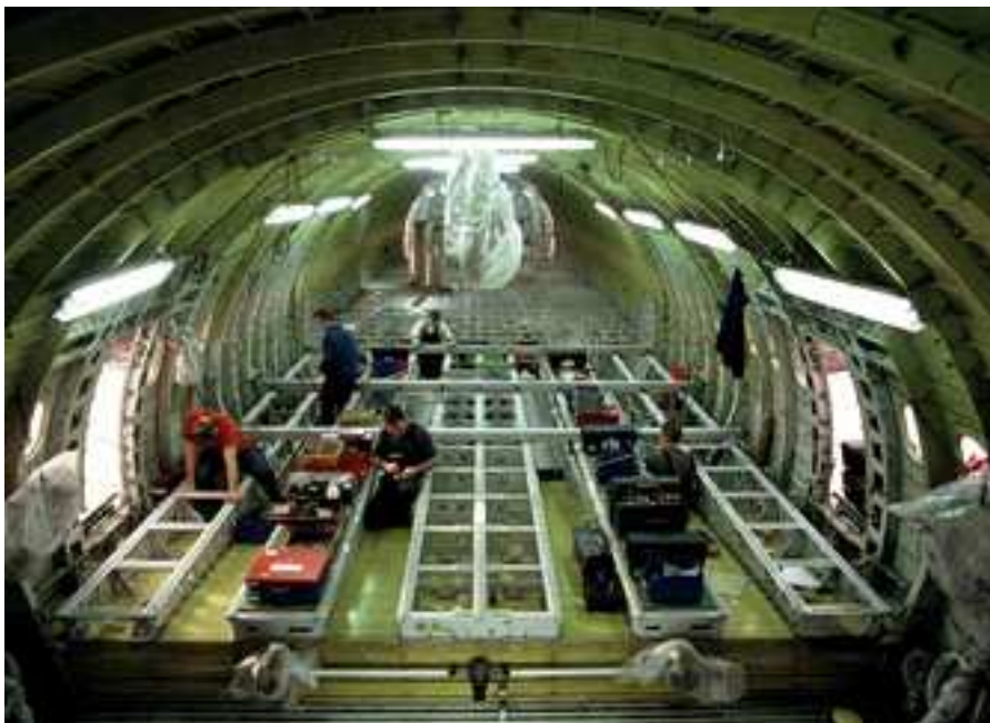
Figure 2.14 Freightier Conversion of an A300 (EADS 2009)
