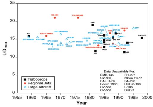
Fig.3.6 Aerodynamic data for commercial aircraft: L/D for cruise (Babikian 2001)
