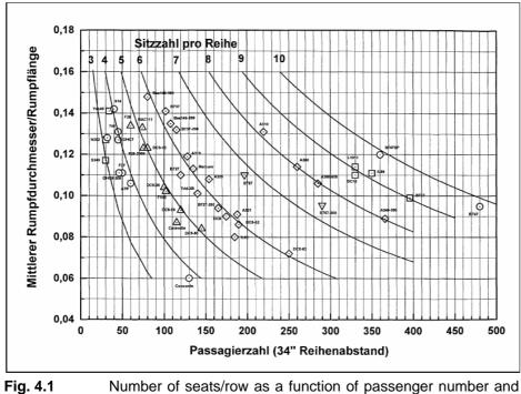
Fig. 4.1 Number of seats/row as a function of passenger number an slenderness (Markwardt 1998)
