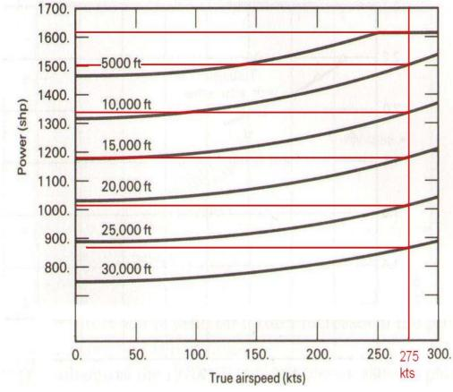
Fig.3.6 Maximum Cruise Power for the PW 120 turboprop, (McCormick 1995)
