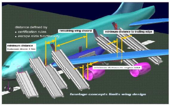
Fig. 5.3 The fuselage concepts limits the wing design (Böttger 2008)
