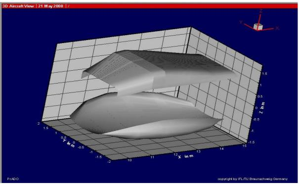
**Fig. 10.10** Undercarriage fairings for the landing gear integration and wing fairings for wing integration designed with PRADO – 2 (**Domingues 2008**)
