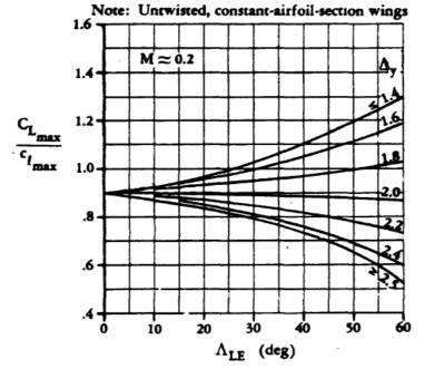
Fig. 6.5 Maximum lift of tapered wings with a high aspect ratio in subsonic speeds (DATCOM 1978)
