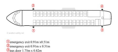
Fig. 4.5 Emergency exit locations and dimensions (sample seating configuration) (www.aviation-safety.net 2008)
