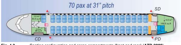
Fig. 4.3 Seating configuration and cargo compartments (front and rear) (ATR 2008)
