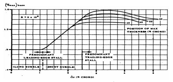
**Fig. 6.4** Maximum lift coefficient of an airfoil, at  $9 \cdot 10^6$  Reynolds number (**DATCOM 1978**)
