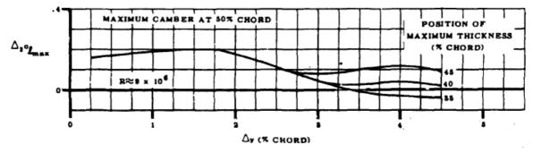
Fig. 6.3 Diagram for correction term for the position of maximum thickness (DATCOM 1978)
