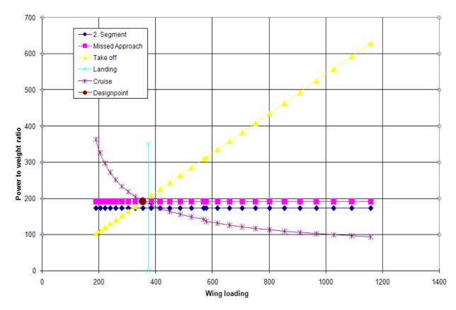
Fig. 3.9 Matching chart for the preliminary sizing of the ATR 72
