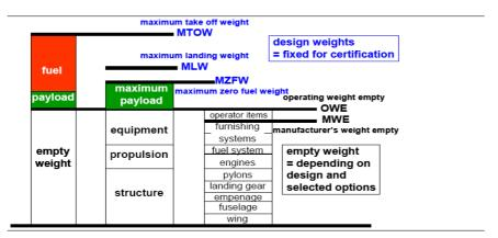
Fig. 8.1 Weight Break Down (Trahmer 2008)
