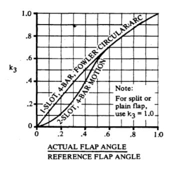
Fig. 6.8 Flap motion correction factor (DATCOM 1978)
