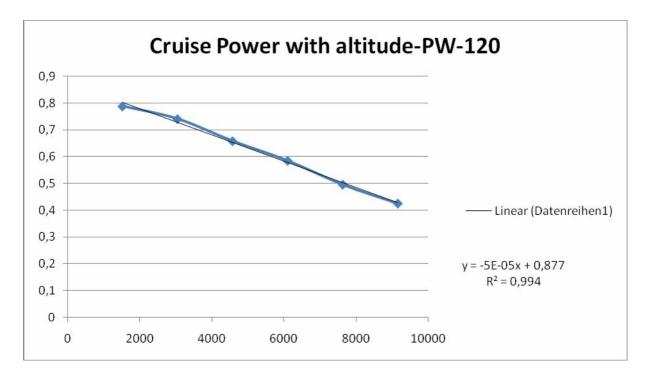
Fig. 3.7 The variation of Cruise Power with altitude for PW 120 turboprop
