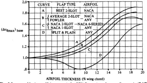
The value is:  $(\Delta c_{L,\text{max}})_{base} = 1.65$  for a thickness of 14%, which is the average thickness.
