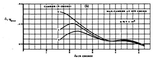
**Fig. 6.2** Diagram for correction term  $\Delta_1 c_{L,max}$  when camber airfoil and position of maximum camber are considered (**DATCOM 1978**)
