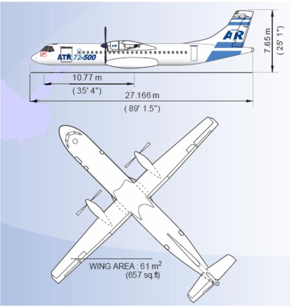
Fig. 2.3b The main parameters of the ATR 72 (ATR 2008)
