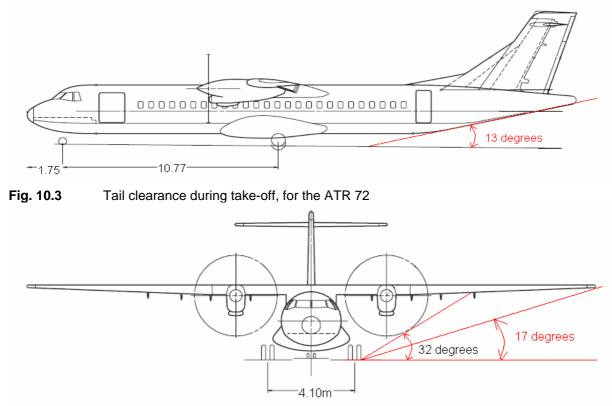
Fig. 10.4 Lateral clearance when one engine fails, for the ATR 72
