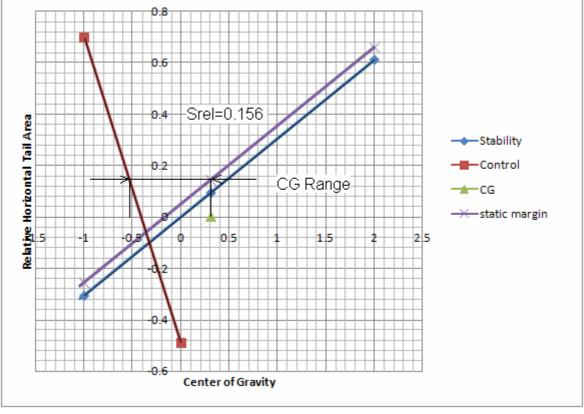
Fig. 9.3 Diagram to determine the minimum required relative horizontal tail area
