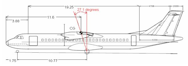
Fig. 10.5 Turn over angle in x-axis direction
