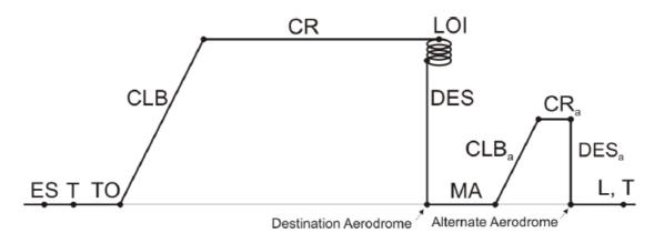
Fig. 3.10 Typical flight phases of a civil transport flight mission
