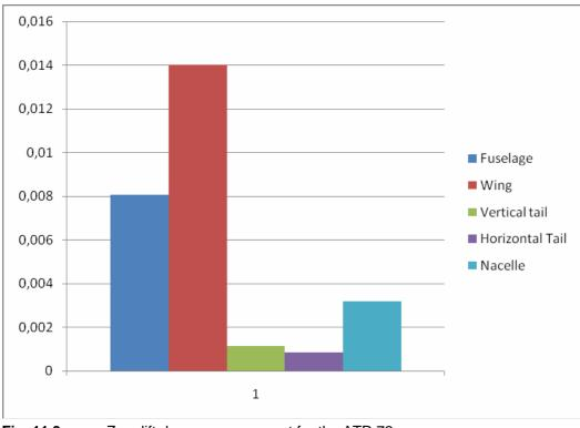
Fig. 11.3Zero lift drag per component for the ATR 72
