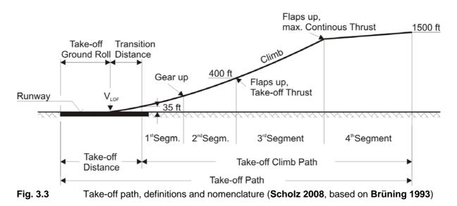
During climb, the thrust T must overcome the drag and also a fraction of the weight, due to climb angle  $\gamma$ . The sum of the forces affecting the aircraft in this case becomes:
