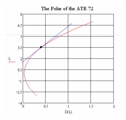
Fig. 11.6 The polar of ATR 72 calculated with statistical Oswald factor
