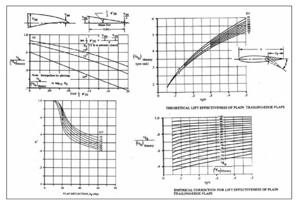
Fig. 9.3 Parameters for the Vertical Tailplane Sizing (DATCOM 1978)
