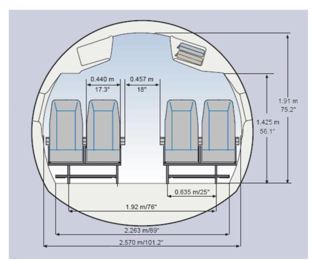
Fig. 4.2 Cross Section view and dimensions (ATR 2008)
