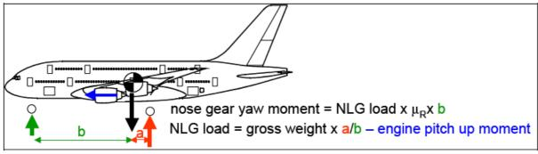
Fig. 10.6 Nose gear load drivers (Trahmer 2008)
