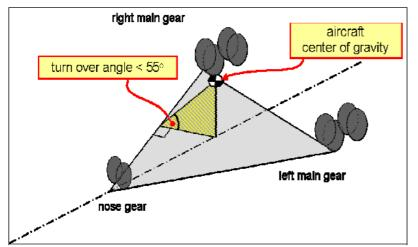
Fig. 10.1 Landing gear position, so to prevent lateral turn-over (Trahmer 2008)
