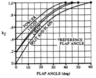
Fig. 6.7 Flap angle correction factor; the reference values are marked by dots (DATCOM 1978)
