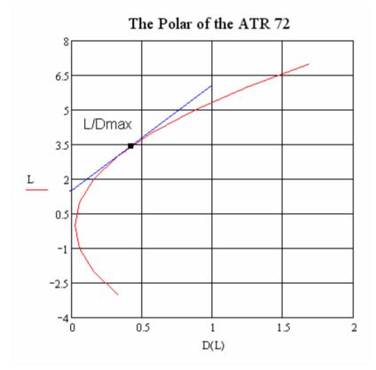
Fig. 11.5 The polar of the ATR 72, representing equation (11.2.7), with calculated Oswald factor
