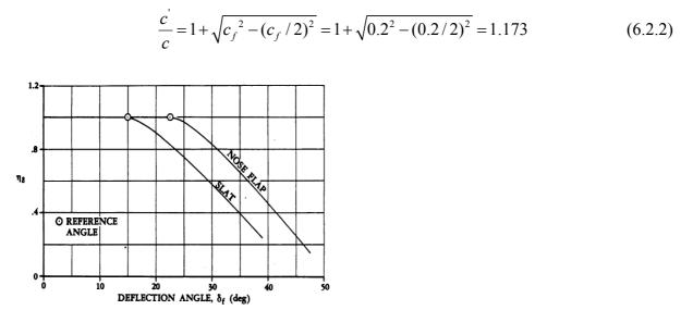
Fig. 6.11 Empirical factor accounting for the real deflection factor in contrast to the reference angle (DATCOM 1978)
