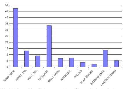
Fig. 11.1 Zero lift drag caused by various parts of a typical transport aircraft (Böttger 2008)
