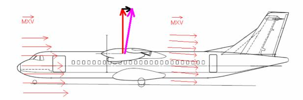
Fig. 11.4 The lift and drag on the ATR 72
