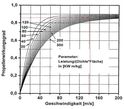
Fig.3.8 Propeller Efficiency Diagram (Scholz 2000)
