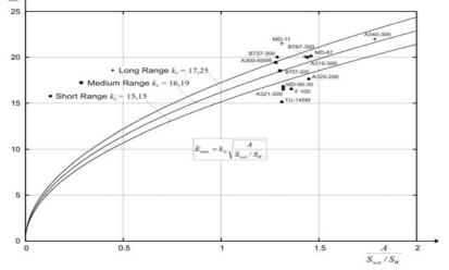
Fig. 3.4 Estimation of glide ratio, wetted area and wing area (Raymer 2006)
