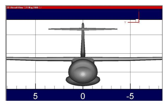
**Fig. 10.9** Undercarriage fairings for the landing gear integration and wing fairings for wing integration designed with PRADO – 1 (**Domingues 2008**)
