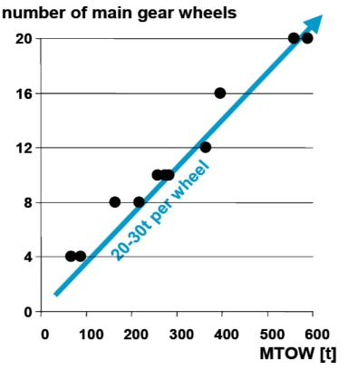
Fig. 10.7 Empirical diagram of number of wheels vs MTOW (Trahmer 2008)
