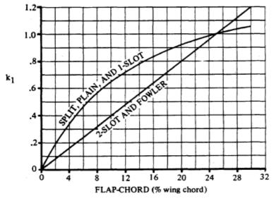
**Fig. 6.6** Flap chord correction factor,  $k_1$  (**DATCOM 1978**)
