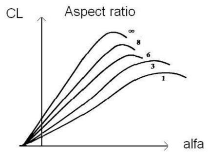
Fig. 5.5 Effect of aspect ratio on lift curve slope (Raymer 2006)
