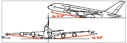
Fig. 10.2 Tail clearance and bank clearance angle (Trahmer 2008)
