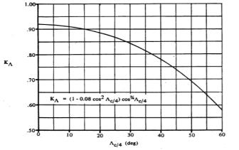
Fig. 6.10 Correction factor that takes the sweep into account (DATCOM 1978)
