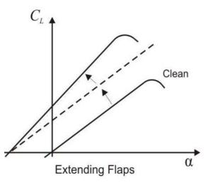
Fig. 6.1 Comparison of lift curves in the case of extending flaps with the clean wing (Raymer 2006)
