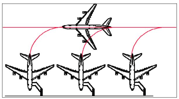
Fig. 5.2 Aircraft span limited by airport requirements (Scholz 2007)
