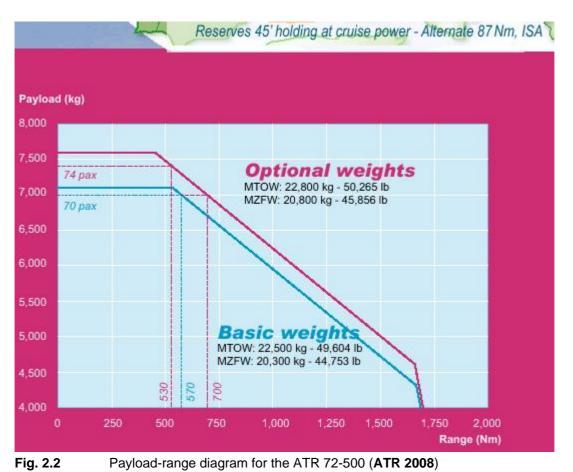
In our design we will define a payload range diagram for a passenger weight of 95kg; the design range will be 800NM, for 70 passengers (so a payload of 6650kg)
