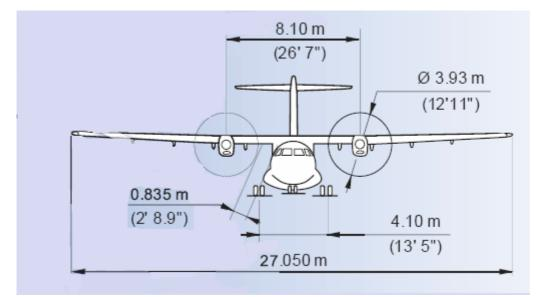
Fig.2.3a The main parameters of the ATR 72 (ATR 2008)
