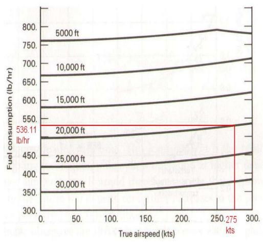
**Fig.3.10** Fuel Consumption with airspeed for the PW 120 (**McCormick 1995**) We can extract from the graph the fuel consumption for cruise; by dividing to power we obtain the specific fuel consumption:
