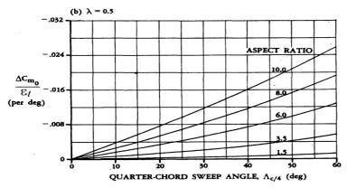
Fig. 9.2 Influence of linear wing twist on pitching moment coefficient with respect to the wing aerodynamic center (DATCOM 1978)
