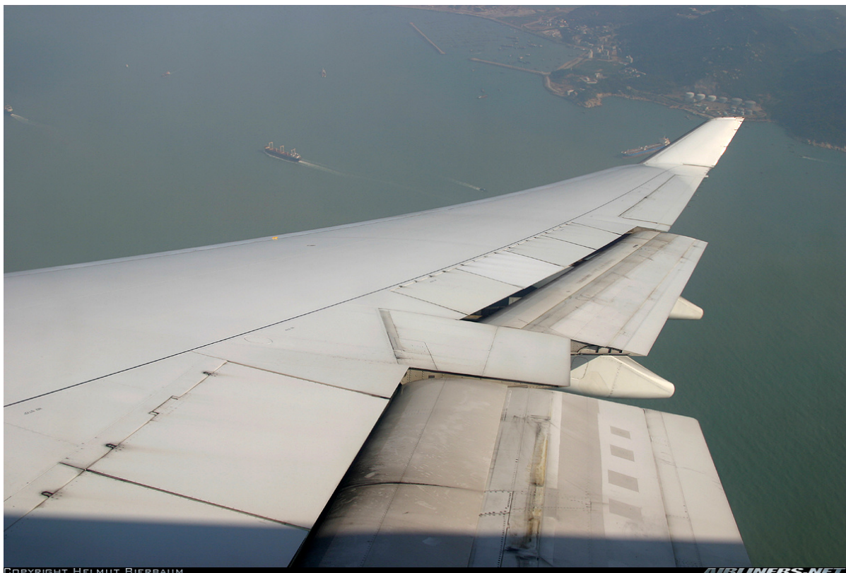
Figure 2.2: Extended Flaps during Landing ( Airliners 2008 )
