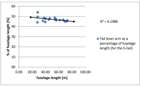
**Figure 3.9** Tail lever arm as a percentage of the fuselage length (for the horizontal tail) – Category A
