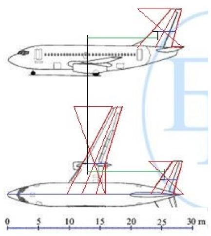
Figure 3.6 Boeing 737-100 side and top view (Roux 2012)
