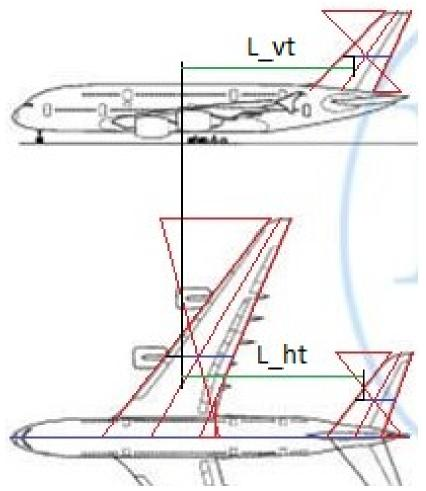
**Figure 3.4** Graphical determination of  $L_{VT}$  and  $L_{HT}$  on the Airbus A380 (based on **Roux 2012**)
