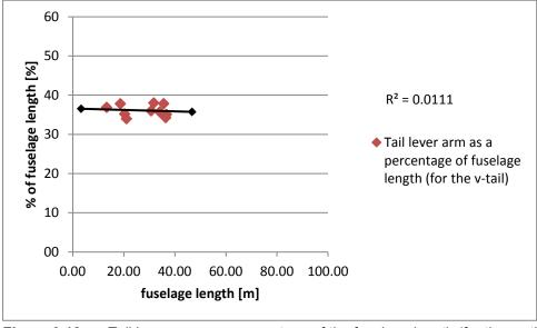
Figure 3.12 Tail lever arm as a percentage of the fuselage length (for the vertical tail) – Category B
