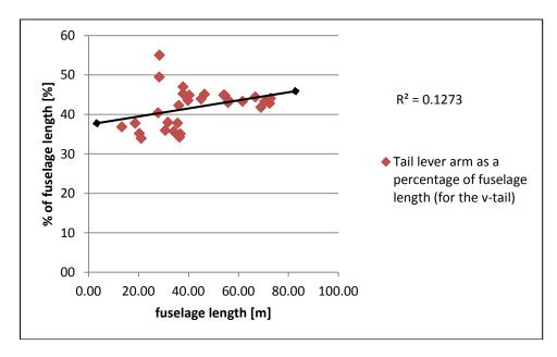
Figure 3.8 Tail lever arm as a percentage of the fuselage length (for the vertical tail)
