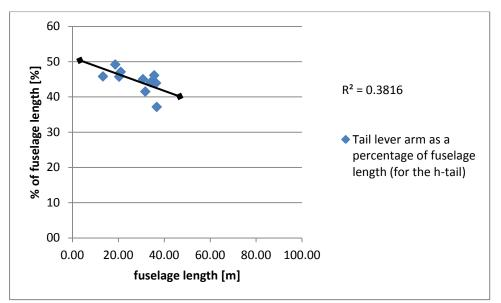
Figure 3.11 Tail lever arm as a percentage of the fuselage length (for the horizontal tail) – Category B
