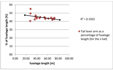
**Figure 3.10** Tail lever arm as a percentage of the fuselage length (for the vertical tail) – Category A
