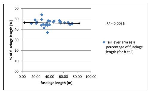
Figure 3.7 Tail lever arm as a percentage of the fuselage length (for the horizontal tail)
