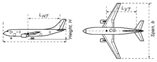
Figure 2.1 Geometric parameters for the tail volume coefficients
