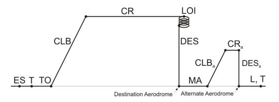
Figure 4.4 Typical flight phase of a civil aircraft flight mission (Scholz 2015).
