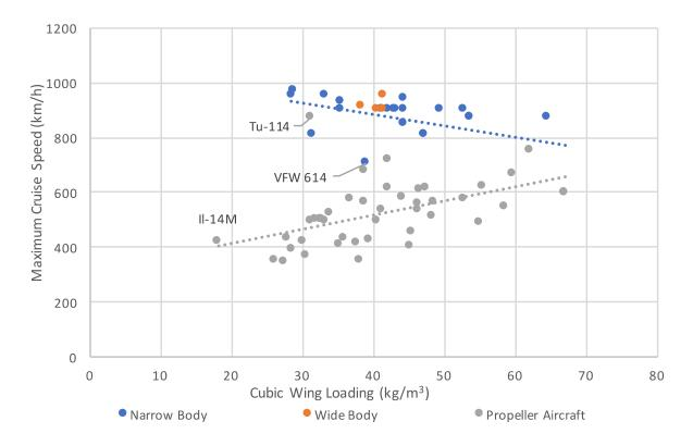
Figure 5.9 Maximum Cruise Speed and Cubic Wing Loading.
