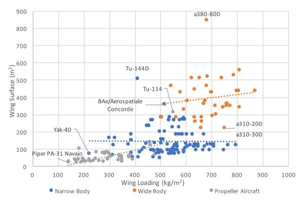
Figure 5.4 Wing Surface and Wing Loading.
