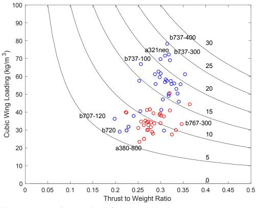
Figure 6.3 Performance Factor for Airbus and Boeing's models.
