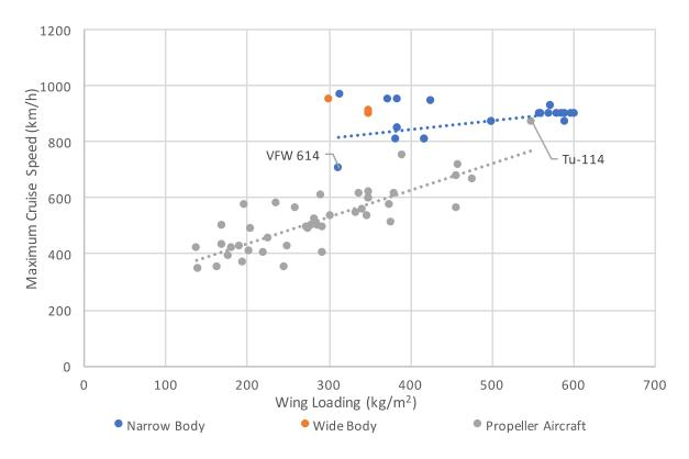
Figure 5.10 Maximum Cruise Speed and Wing Loading.
