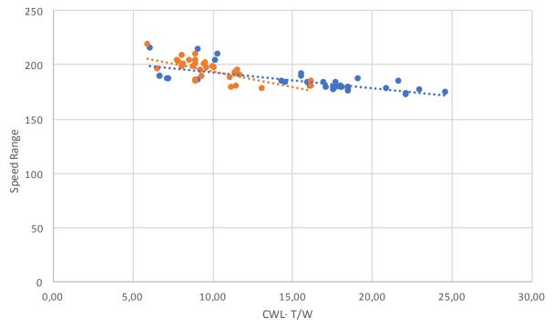
Figure 6.2 Speed Range and Performance Factor for 72 Airbus and Boeing's models (CWL·T/W).
