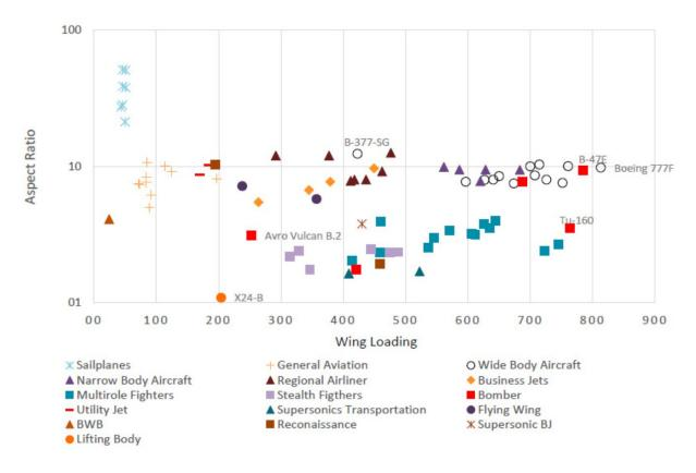
**Figure 2.7** Aspect ratio and wing loading chart of 81 aircraft. A base 10 log. Scale for AR was used for the readability of the scatter plot. (Durmus 2020)
