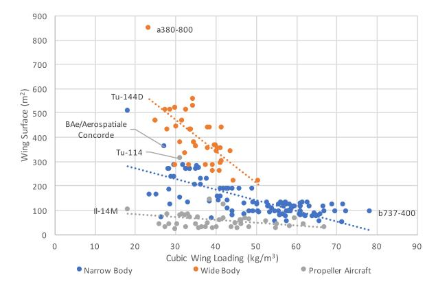
Figure 5.3 Wing Surface and Cubic Wing Loading.
