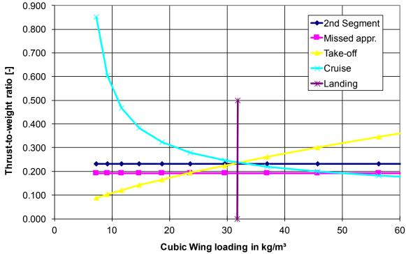
Figure 4.2 Matching chart. Lines mark restrictions as imposed by equations.
