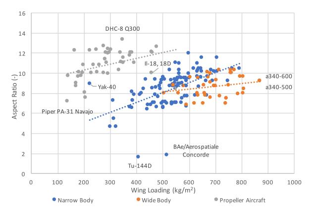
Figure 5.6 Aspect Ratio and Wing Loading.
