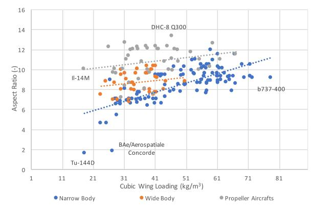
Figure 5.5 Aspect Ratio and Cubic Wing Loading.
