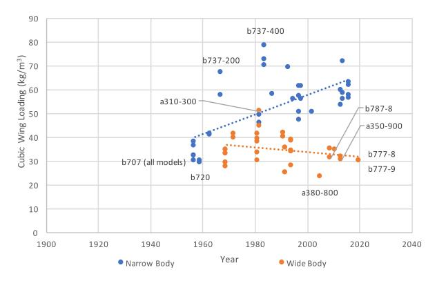
Figure 5.13 Cubic Wing Loading through Years.
