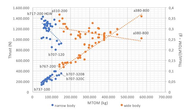
**Figure 6.9** T versus  $m_{MTO}$  (MTOM) and T/( $m_{MTO}$ ·g) =T/W (T/(MTOM·g)) lines.
