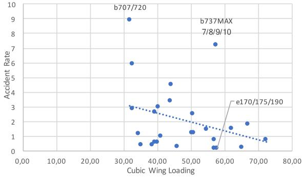
Figure 6.5 Accident Rate over Cubic Wing Loading.
