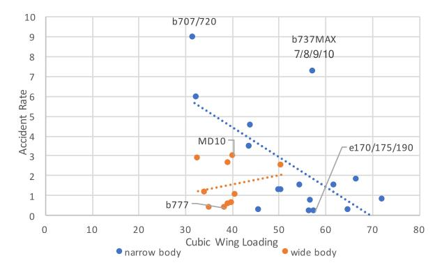
Figure 6.6 Accident Rate over Cubic Wing Loading for narrow-body and wide-body aircraft.
