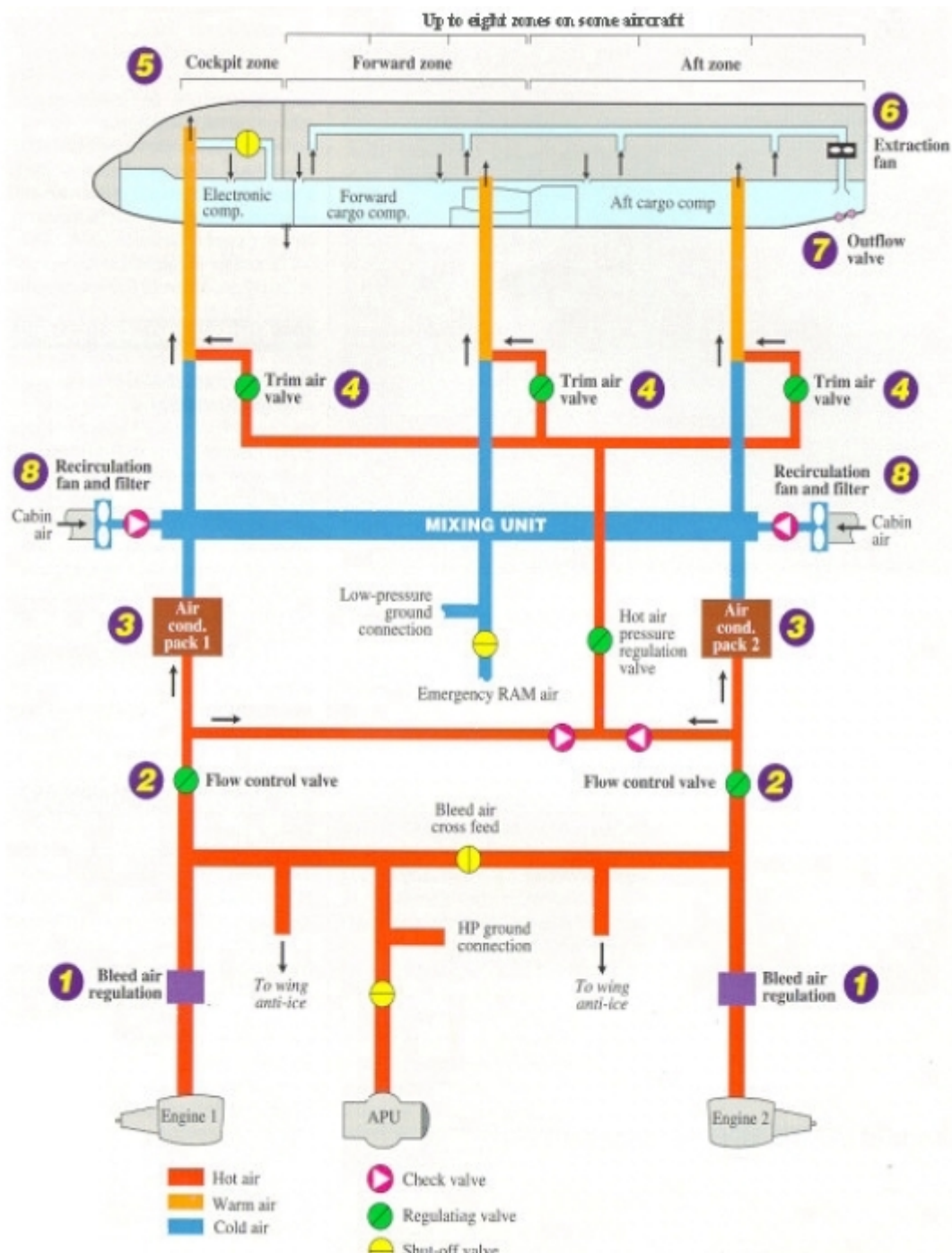
Figure 4.1: A321 air conditioning system structure
