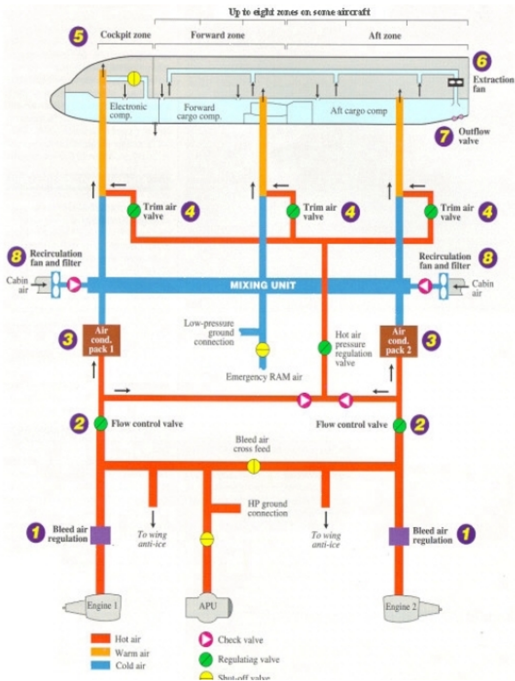
Figure 2.1: Airplane air conditioning system structure example and main components Regulation temperature systems:
