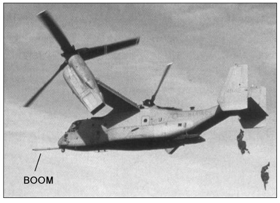
Fig.: 10-5 The Boeing Osprey with nose boom (FLUGREVUE)
