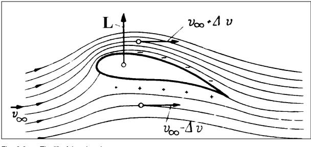
Fig.: 3-9 The lift of the wing shape (Schlichting 1967 p. 83)
