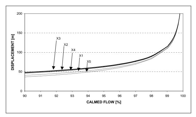
Fig.: 3-7 The calmed flow besides the fuselage over the displacement in x-steps
