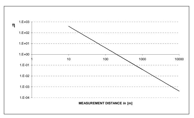
Fig.: 17-8 The measurement distance due to  $\eta$  in the height of 45000 ft
