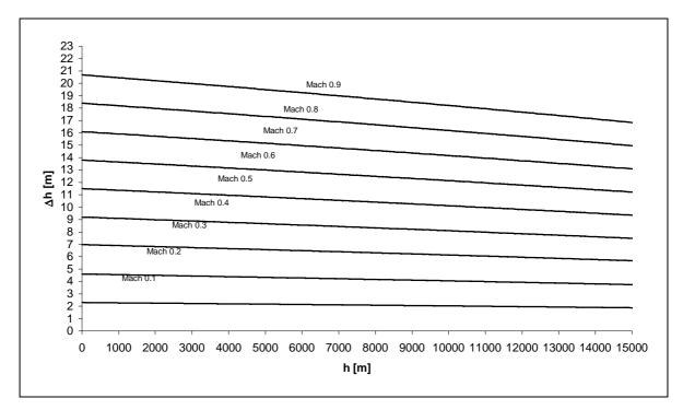
Fig.: 7-2 The altitude error of the I.C.A.O. over the height and Mach number
