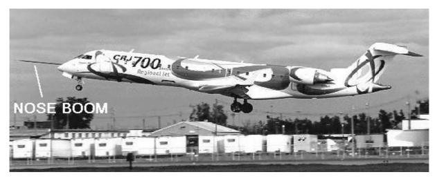
Fig.: 10-6 The Bombardier CRJ700 with nose boom (FLUGREVUE)
