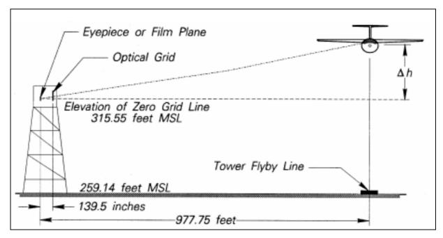
Fig.: 8-2 The tower fly-by calibration method (Ward 1993)
