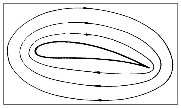
Fig.: 3-10 The circulation of the wing shape (Schlichting 1967 p. 83)
