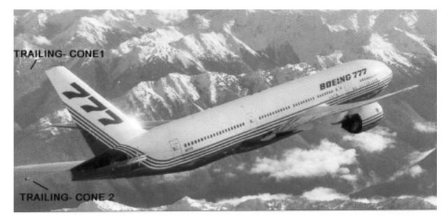
Fig.: 10-4 The Boeing 777 with two different trailing-cones (FLUGREVUE)
