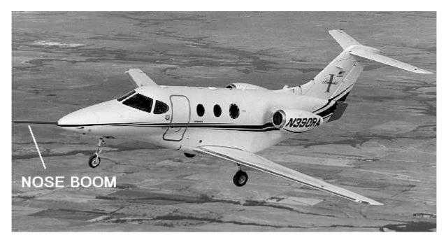
Fig.: 10-11 The Raytheon Aircraft's Premier with nose boom (FLUGREVUE)
