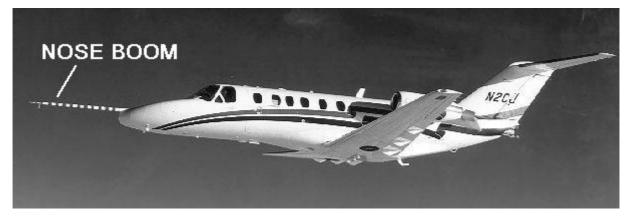
Fig.: 10-7 The Cessna Citation CJ2 with nose boom (FLUGREVUE)
