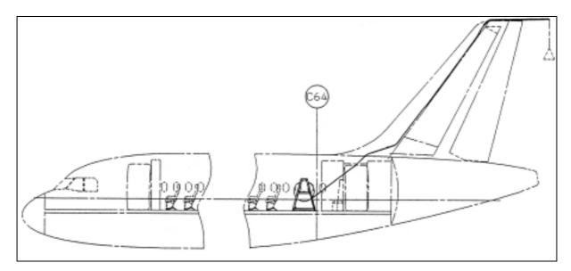
Fig.: 9-1 The trailing cone on Airbus (ETF)
