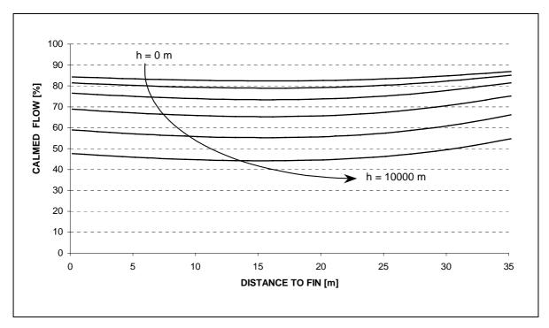
Fig.: 13-1 The calmed flow over distance to fin in variable height (Mach 0,3)
