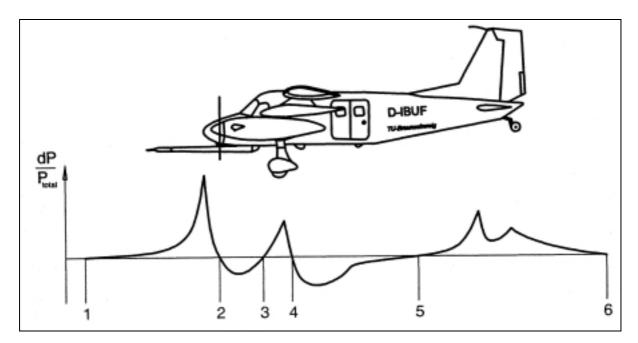
Fig.: 8-1 The computed position error on the DO 128 (Delft 1999)
