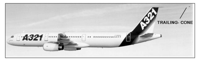
Fig.: 8-4 The trailing cone calibration method on the A321 (Airbus)
