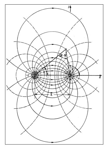
Fig.: 3-5 The source lowering flow (Schlichting 1967 p. 64)
