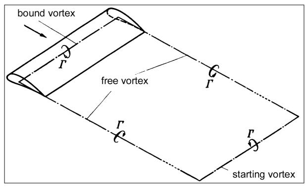
Fig.: 3-11 The circulation of the wing with finite span (Schlichting 1967 p. 92)
