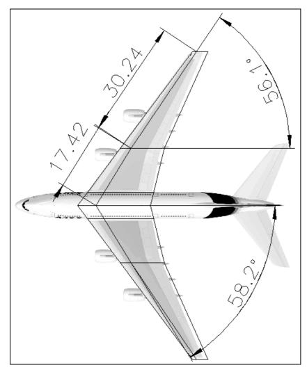
Fig.: 3-12 The simple geometry of the A3XX wing
