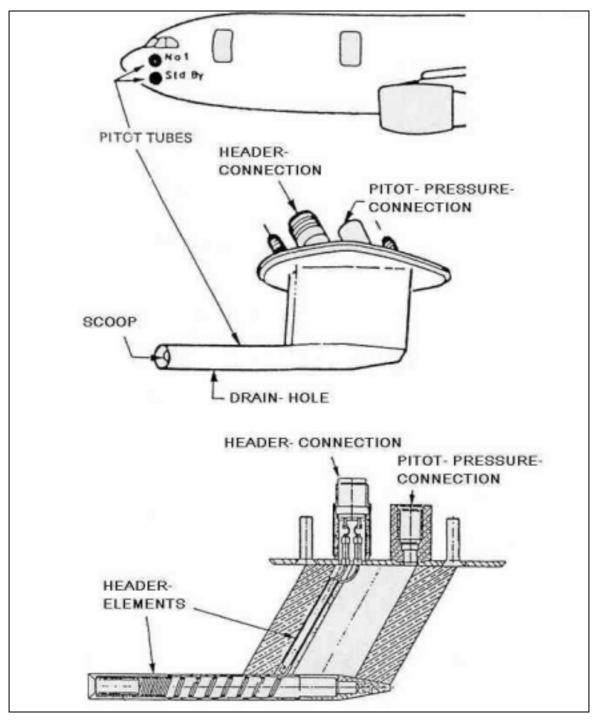
Fig.: 4-1 The pitot tube on aircraft (Bräunling)
