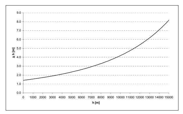
Fig.: 7-4 The altitude error of the calibration equipment
