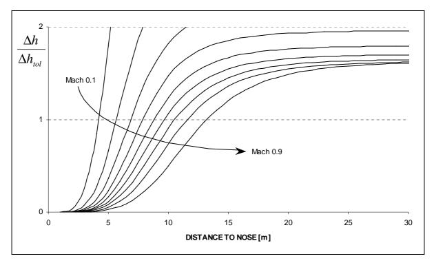
Fig.: 17-4 The height error relation over distance to nose (Mach 0,1-0,9) at MSL
