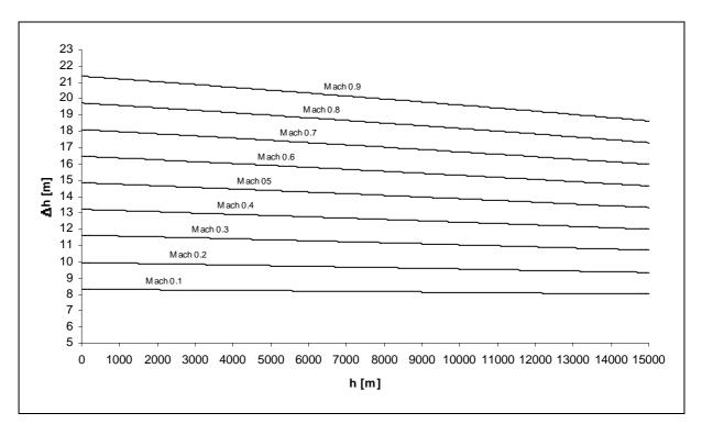
Fig.: 7-4 The altitude error of FAR and I.C.A.O. over the height end Mach number
