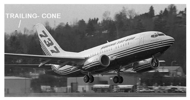
Fig.: 10-1 The Boeing 737-600 with trailing-cone (FLUGREVUE)
