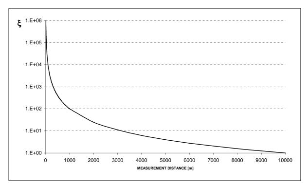
Fig.: 17-7 The distance-ratio over the measurement distance for ODIN-3
