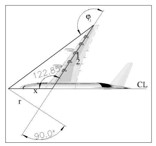
Fig.: 3-13 The circulation geometry for the nose calculation
