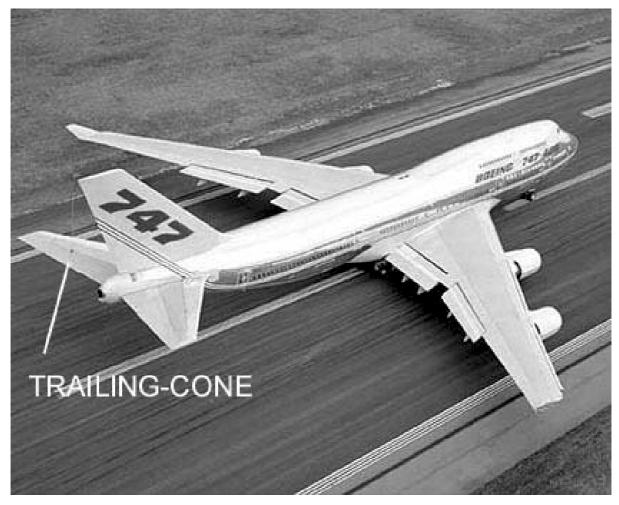
Fig.: 10-2 The Boeing 747-400 with trailing-cone (DISCOVERY)
