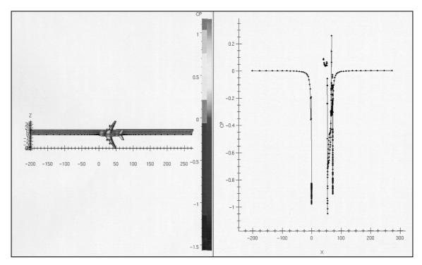
Fig.: 13-7 The pressure coefficient  $c_p$  for the A3XX (**EFD**)
