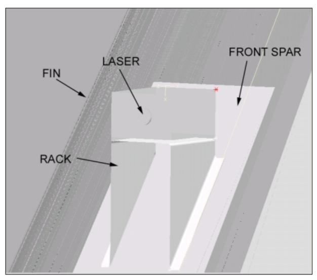
Fig.: 17-12 The laser attached on the front spar of the fin
