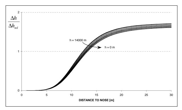
Fig.: 17-5 The height error relation over distance to nose in steps of 2000 m (Ma 0,9)
