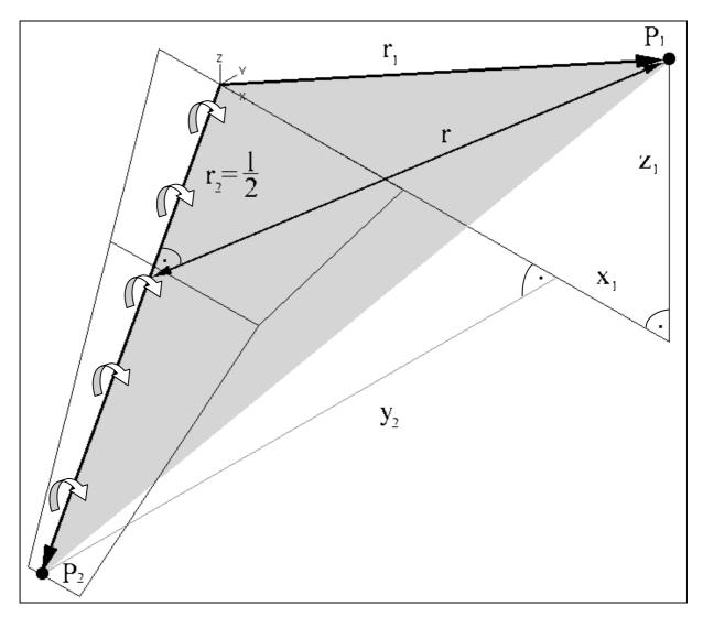
Fig.: 3-14 The circulation geometry of the calculation above the fuselage (CL)
