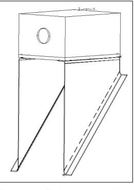
Fig.: 17-11 The laser rack assembly
