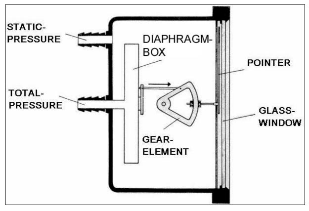
Fig.: 5-5 The analog airspeed indicator (Götsch 1989)
