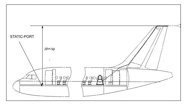
Fig.: 12-1 The trailing cone direct measurement (ETF)
