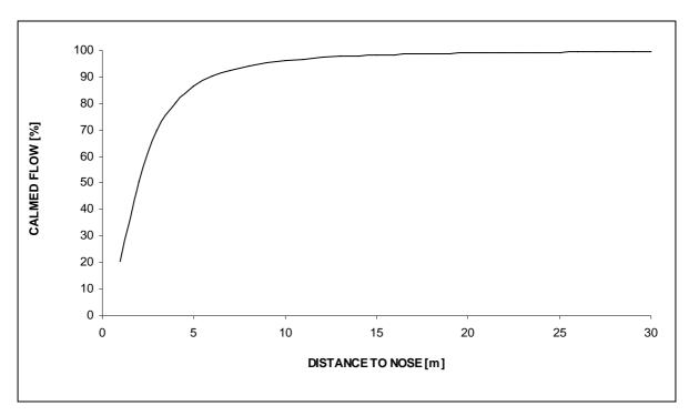
Fig.: 13-4 The calmed flow over distance to nose
