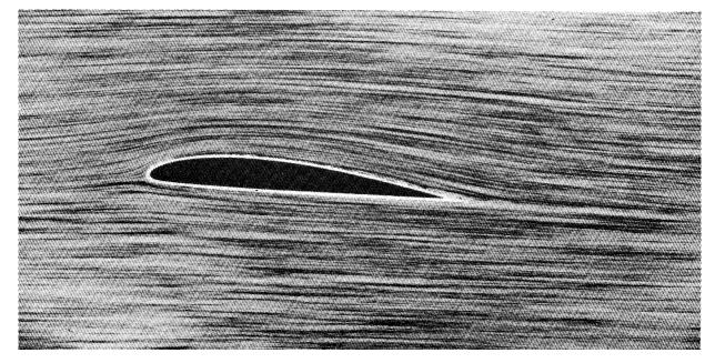
Fig.: 3-3 The displacement on a wing shape (Schlichting 1967 p. 257)
