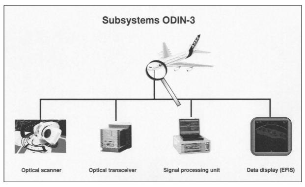
Fig.: 17-2 The subsystems of ODIN-3 (Kayser)
