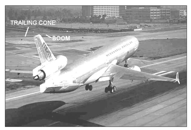
Fig.: 10-10 The Mc Donnell Douglas MD 11 with trailing-cone and boom (FLUGREVUE)
