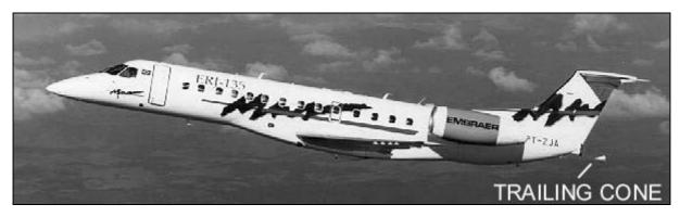
Fig.: 10-9 The Embraer ERJ 135 with trailing-cone (FLUGREVUE)
