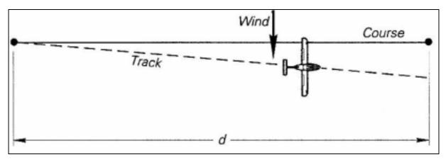
Fig.: 8-6 The speed-course calibration method (Ward 1993)
