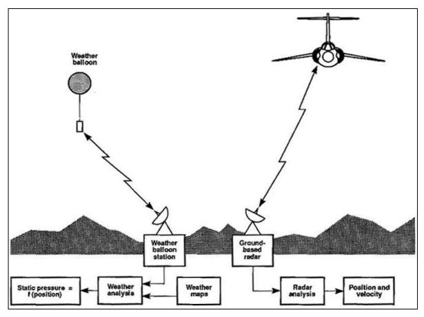
Fig.: 8-3 The radar tracking method (AGARD 1995)
