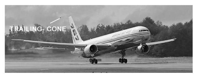
Fig.: 10-3 The Boeing 767-400 with trailing-cone (FLUGREVUE)
