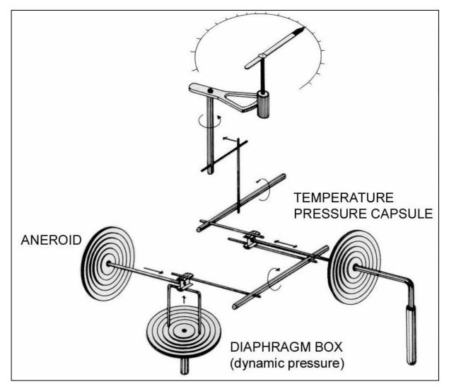
Fig.: 5-6 The analog compensating airspeed indicator (Götsch 1989)
