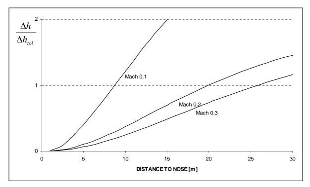
Fig.: 17-3 The height error relation over distance to nose (Mach 0,1-0,3) at MSL
