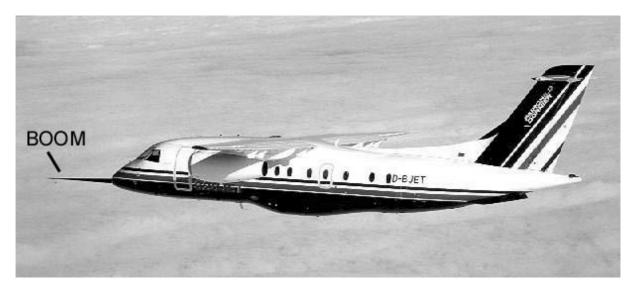
Fig.: 10-8 The Dornier Fairchild 328 Jet with nose boom (FLUGREVUE)
