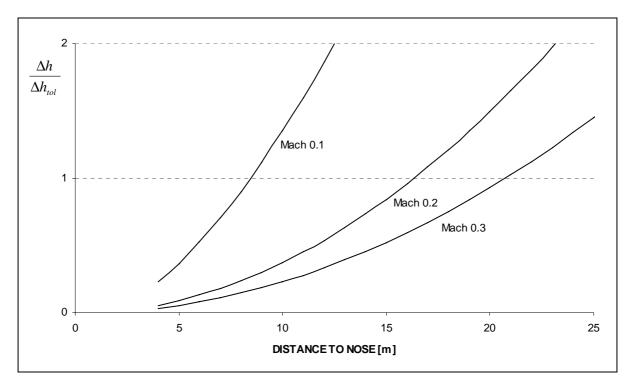
Fig.: 13-6 The height error relation over distance to fin (Mach 0,1–0,3)
