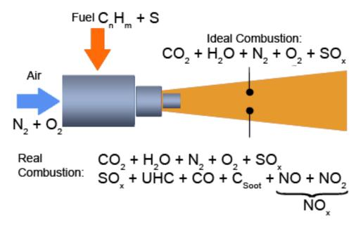
Figure 3.4 Combustion products of a jet engine (adapted from Norman et al. 2003)
