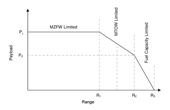
Figure 4.2 Schematic payload/range diagram
