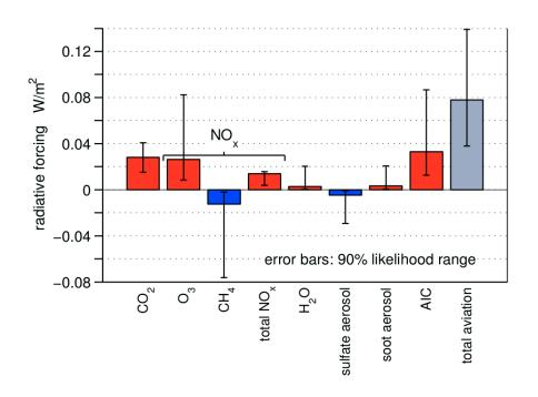
Figure 3.9 Radiative forcing components of aviation emissions (Schwartz 2011, based on Lee et al. 2009)
