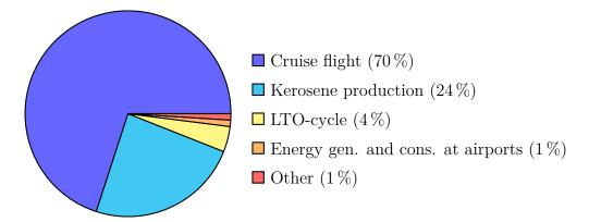
Figure 3.2 Environmental impact of processes of an Airbus A320-200 using LCIA (Johanning 2014)
