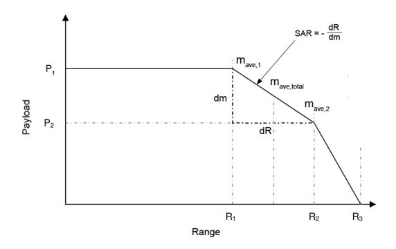
Figure 4.3 Payload/range diagram with SAR
