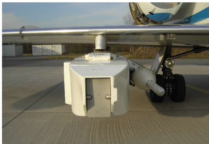
Fig. 5.1 MTR-101 Pod installed under the wing of a Learjet 35A/36A
