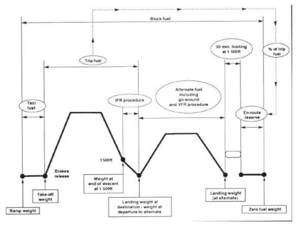
Fig. 6 Fuel Plan (example: Standard Fuel Plan) [2]
