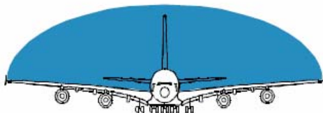
Figure 2.16 Difference between aerodynamic and weight optimal lift distribution (Böttger 2004)
