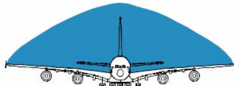
Figure 2.16 Difference between aerodynamic and weight optimal lift distribution (Böttger 2004)
