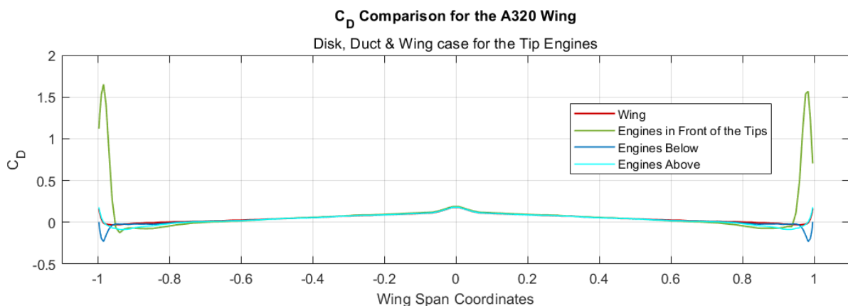
Figure 5.37 Graphical representation of the drag coefficient results of the Tip Engines distributions for the disks, ducts & wing case.
