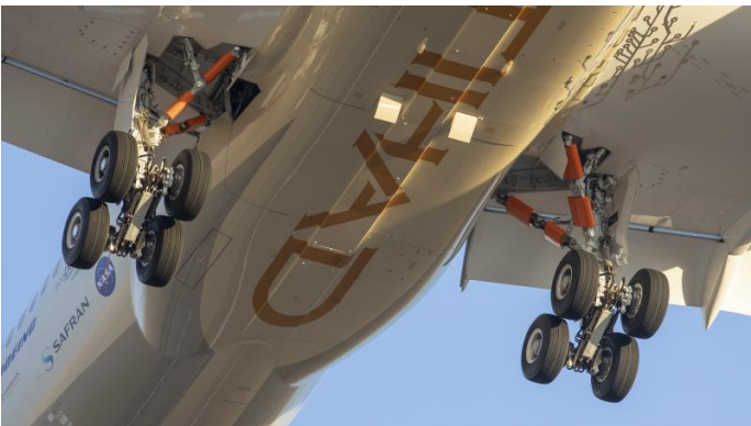
Simple MLG general arrangement
