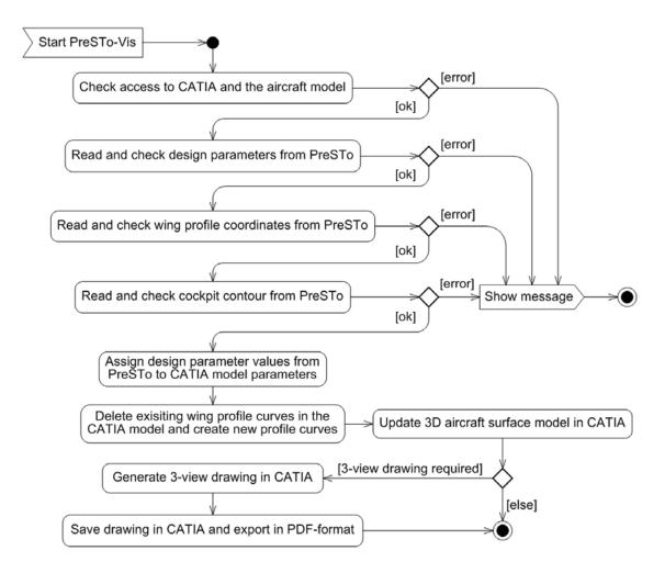
Figure 4: Activity diagram of PreSTo-Vis
