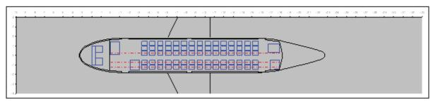
Figure 5: PreSTo cabin floor plan of Fairchild-Dornier 728 re-design
