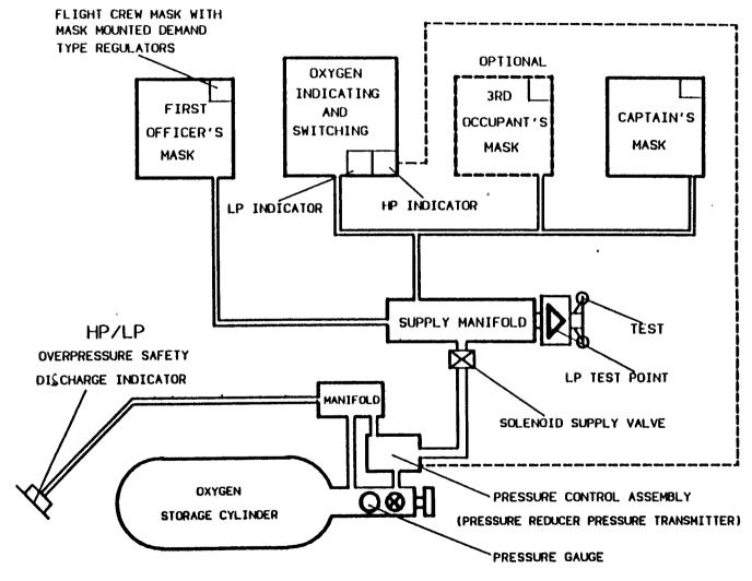
Figure 35-1 Crew Gaseous Oxygen System Schematic
