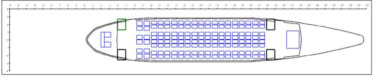
Figure 8.3 Cabin floor plan of the box wing aircraft (modelled with PreSTo Cabin)
