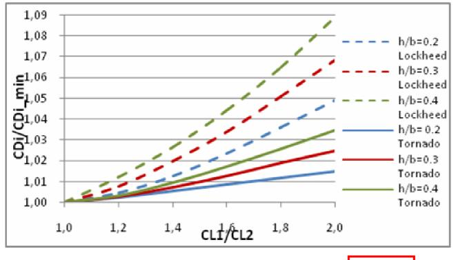
Sensitivity of induced drag to non-optimum lift distributions (Tornado) - Stagger = 0
