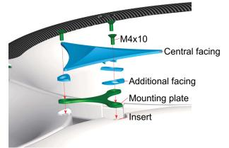
FIG 12. Cell connector between three cells
