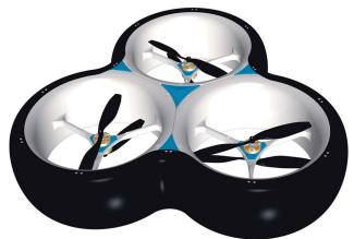
FIG 1. CellDrone made from three cells
