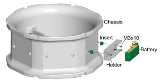
FIG 4. Connection between battery and airframe
