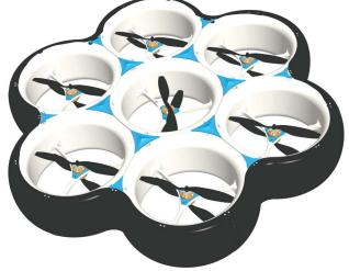
FIG 2. CellDrone made from seven cells
