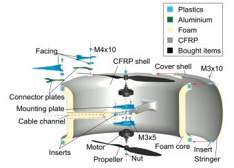
FIG 13. Cross-section of one cell
