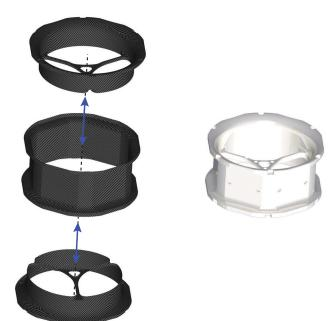
FIG 9. CFRP shell around foam core
