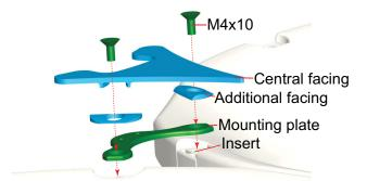
FIG 11. Cell connector between two cells
