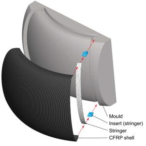
FIG 10. Assembly of the cover shells
