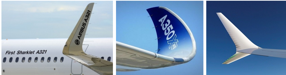
Figure 1: Different winglets on passenger aircraft: A321 Sharklet [1], A350XWB Blended Winglet [2] and B737 MAX AT Winglet [3]
