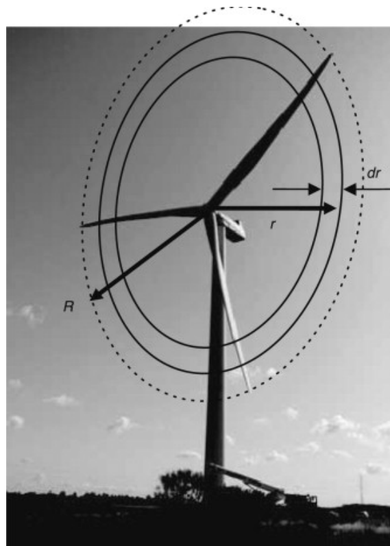
Figure 8. The Blade Element Momentum Theory (BEMT) divides the disc area into several annular rings of width dr at a representative radius, r [2].
