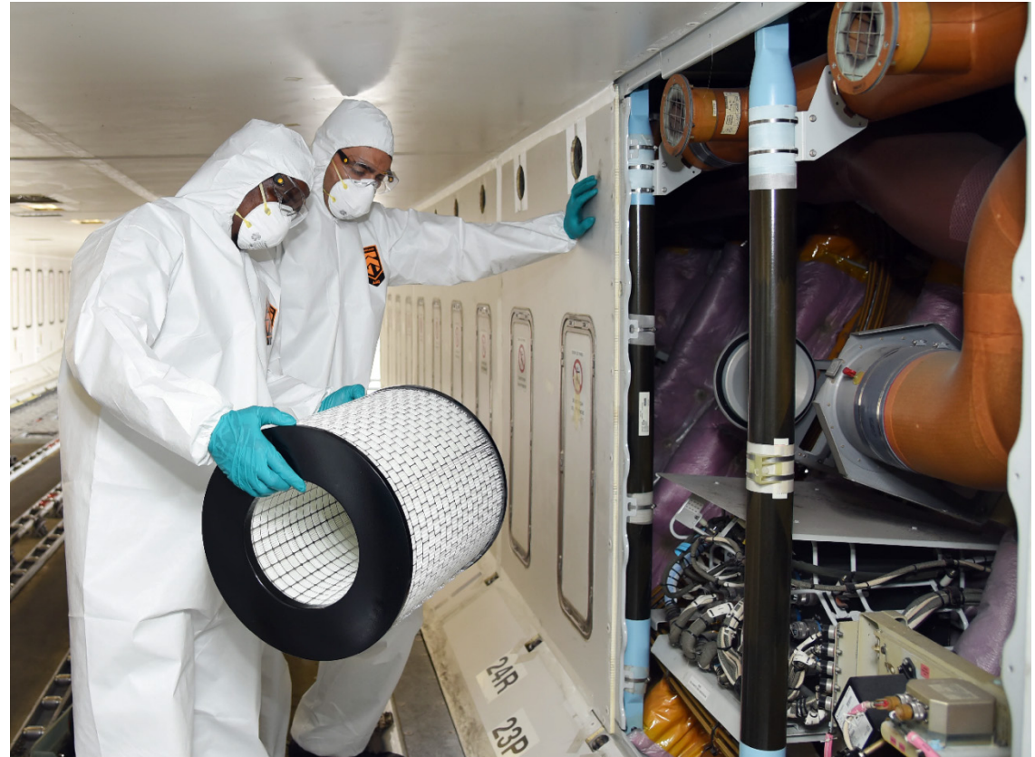
Airbus A380, Emirates. Installing a new HEPA filter. High risk operation?
