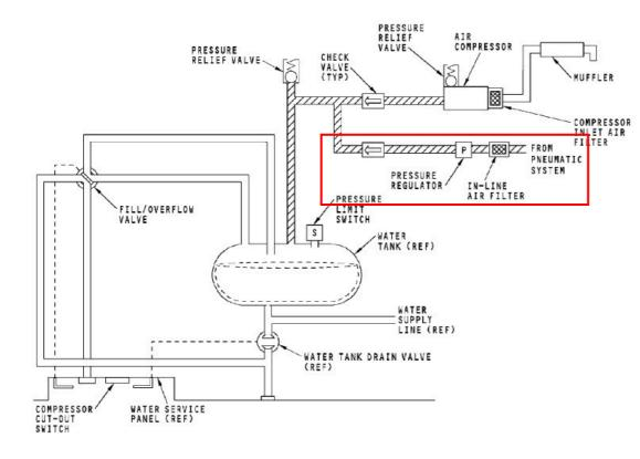
Possible bleed air contaminations could reach the potable water passing a filter and a check valve (in flow direction).
