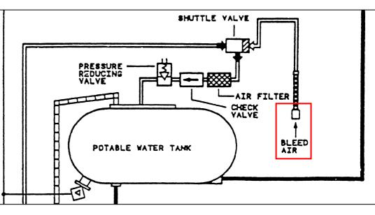
Training Material A320: Potable Water System pressurization.
