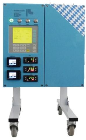
Online analysis system for determination of the THC (Total Hydro Carbon) fraction of the air.
