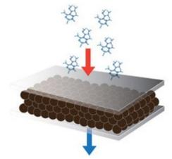
Schematic of carbon Filter (Pall 2011)
