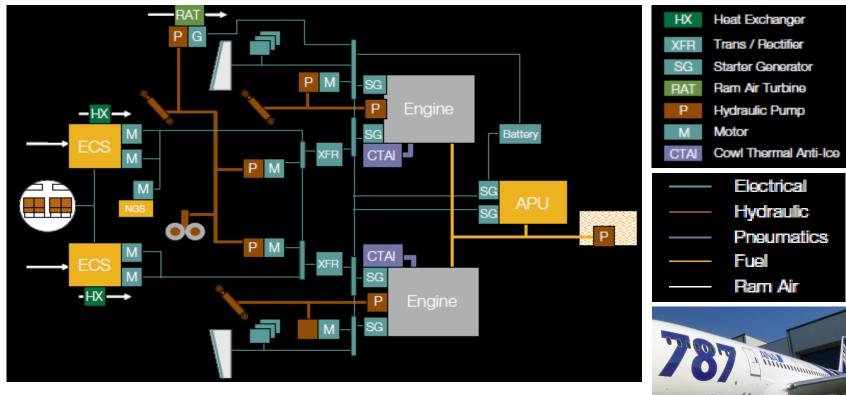
The "Pack" of the B787's Environmental Control System (ECS) is powered by electric motors (M) to compress ambient air up to cabin pressure and to push the air through the heat exchangers (HX) for cooling. The power for the electric motors is produced by generators (SG) connected to the aircraft's engine and APU. After compression and cooling the air is delivered to the cabin.
