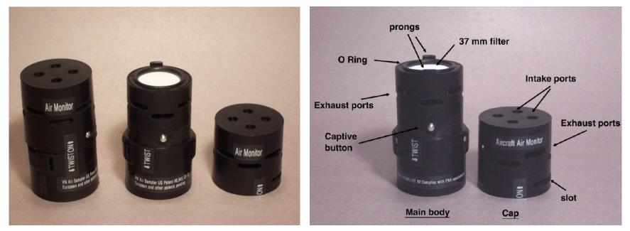
Prof. Van Netten invented this "VN-Sampler". It is <u>not</u> an in situ measurement device, but a means to collect the air in a fume event for later detailed analysis in a laboratory on the ground. The device is FAA approved.
