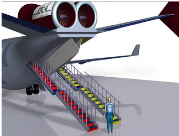
Figure 2.5 Two stairs at the rear of the aircraft (Stuttgart 2008b)
