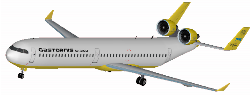
Figure 2.20 Three doors per side and U-Tail (Stuttgart 2008e)
