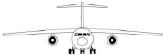
Figure 3.1 Shoulder Wing (Delft 2007)
