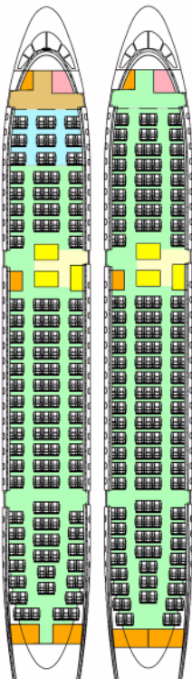
Figure 2.14 Twin-aisle layout (Stuttgart 2008d)
