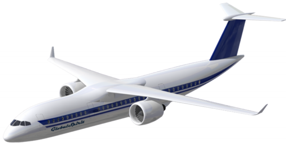
Figure 2.16 Three doors per side and shoulder wing (Stuttgart 2008d)
