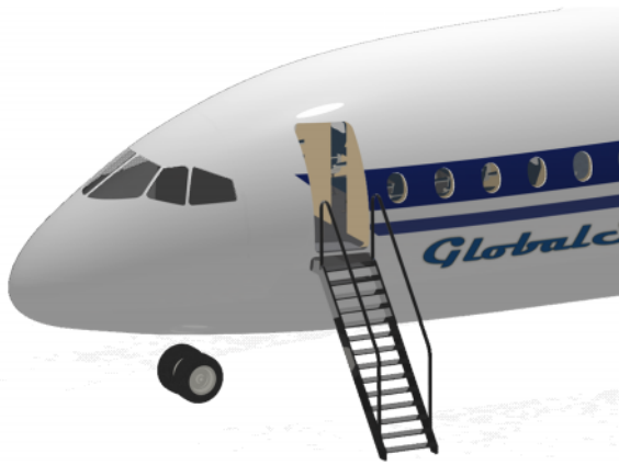
Figure 2.15 On-board stairs (Stuttgart 2008d)
