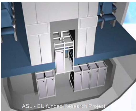
Figure 2.6 Trolley-lift system (Stuttgart 2008b)
