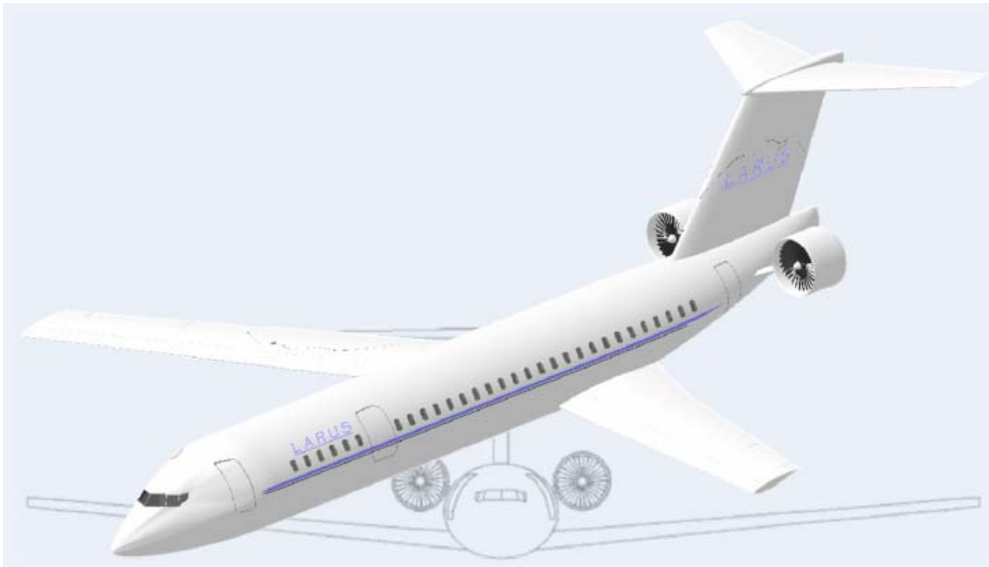
Figure 2.12 Three doors per side and forward-swept wing (Stuttgart 2008c)
